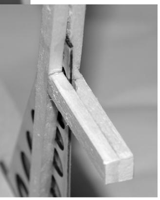
Glue the ply reinforcements and the rudder horn to the rudder. Make sure the rudder horn is centered on the sharp edge, not the centerline.
