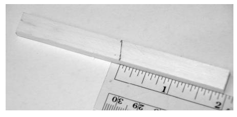
Take the 5x10 mm motor mount block and mark it as shown, 1-15/16" from the end on opposite sides. Draw a line connecting the two marks. Saw the motor mount apart at the line. Glue one of the motor mount sticks to the chassis 5/8" from the top of the plywood part. Glue to the chassis and the mast. Make the angle 75 degrees as shown on the plan. Trim off a little of the other motor mount stick so
