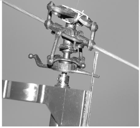
will clear the wheel collar. Once satisfied tighten the set screw on the upper collar. Now push the lower collar up into place against the lower bearings so the whole assembly turns freely but doesn't have any slop.
