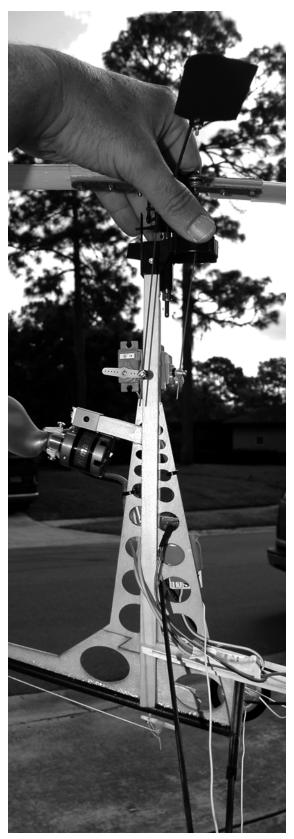
Double check the model over. The controls should move freely. The head should spin freely and not bind. Bend the axles so the main wheels are slightly toed in and cambered out like a good tail dragger should be. Re-check the CG and the trim position of the swashplate.
