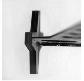
chassis when viewed from the top. Then apply thick CA to the joints and allow to cure.
