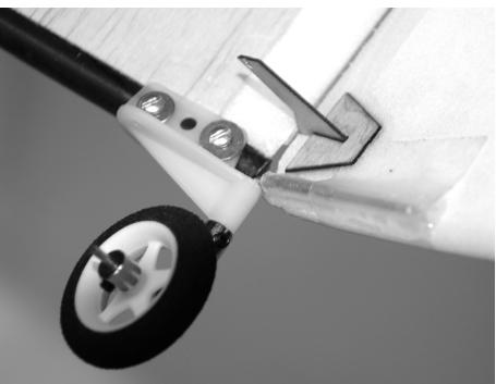
Glue one half of the 2mm wire axles into the ends of the landing gear struts with thick CA. Use part of the kevlar thread (leave some for the head reinforcement later) on each gear leg and wrap the last 1/8" of the gear leg to keep it from splitting. Secure with thin CA. Install the wheels and the 2mm wheel collars. Glue the landing gear struts into the main landing gear blocks.
