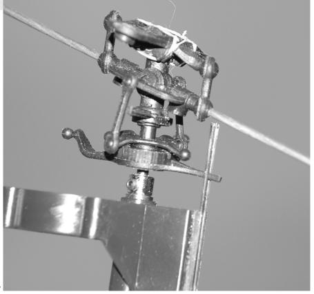
Adjust the upper wheel collar until the bottom of the swashplate is <sup>1</sup>/<sub>2</sub>" from the top of the gearbox. Wiggle the swashplate around to make sure it will clear the wheel collar. Once satisfied tighten the set screw on the upper collar. Now push the lower collar up into place against the lower bearings so the whole assembly turns freely but doesn't have any slop.
