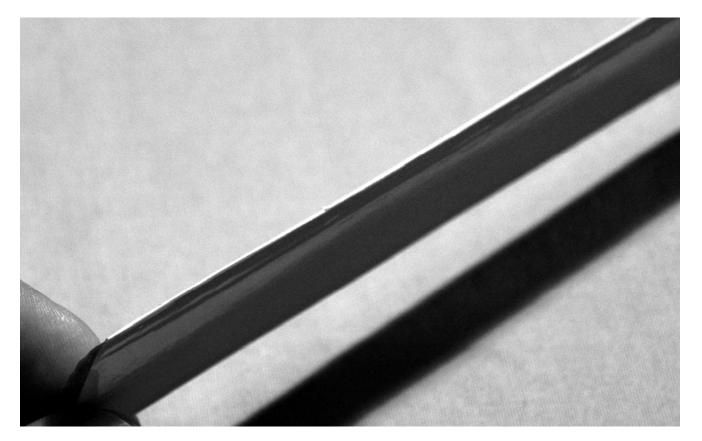
Soak thin CA in the tip and along the edge near the root. If the covering sticks out past the tip, use a sanding block to gently scrub off the excess covering. If you have any bubbles or wrinkles a heat gun can be used carefully to work out some of the problems. Be careful as too much heat will burn a hole quickly. © Copyright 2005, Charles M. Nowell, Jr. 12 All Commercial Rights Reserved.
