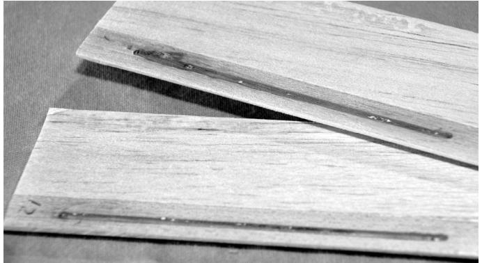
Now sand the blades overall with 220 grit sandpaper. Use a block not your fingers. Wick thin CA down the last 1/8" the whole length of trailing edge. Sand this smooth when cured.
