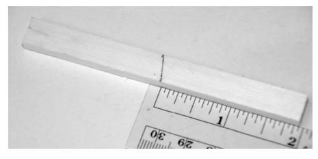
Take the 5x10 mm motor mount block and mark it as shown using the motor mount angle template below, approximately 1-15/16" from the end. Saw the motor mount apart at the line. Glue one of the motor mount sticks to the chassis 5/8" from the top of the plywood part. Glue to the chassis and the mast. Make the angle 75 degrees as shown on the plan. Trim off a little of the other motor mount stick so that it clears
