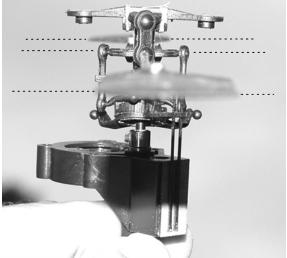
apply some thick CA and sand out until the gearbox has absolutely no wobble on the main mast. If the gearbox wobbles on the mast you
