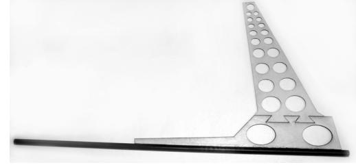
the remaining mast pieces. Place the second mast piece in place and press the whole thing together. Apply accelerator if necessary. You should end up with the mast glued in place on the chassis, to the tail boom and to itself above the chassis.
