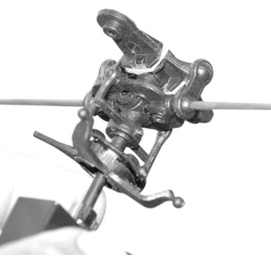
Put on the flybar plate (set screws down) and slide the flybar in place. Make sure that it is centered (use a caliper if you have one) and
