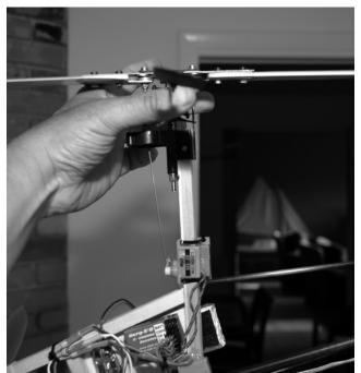
until the nose comes down 1 or 2 degrees from the previous position. In other words you want the main mast to just past vertical in the nose down direction.
